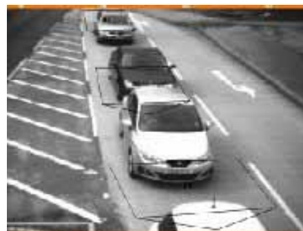
Video images from the TrafiCam sensors with direction sensitive virtual loops
